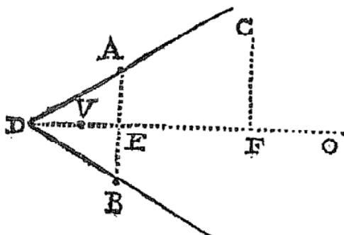
**S**int puncta illa data A, B, C, Tangentes AD, BD ad puncta A & B, D communis intersectio tangentium. Biseca AB in E. Age DE, & produc eam donec in F occurrat CF actæ parallelæ AB: & erit DF diameter, & AE, CF ordinatim applicatae ad diametrum. Produc DF ad O, & in DO cape OV medium proportionale inter DO & EO,
