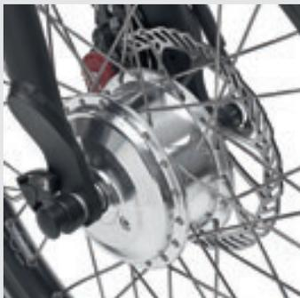
**Electric Motor:** The power pack For long and hilly commutes or just a little extra speed and comfort: the Protanium motor transforms the LEPUS into a trike hybrid. The 250 W package on the front wheel powers along when you start pedaling. Otherwise it travels – incognito – in hub disguise.
