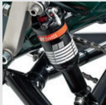
**DT-Swiss shock:** Float like a butterfly ... The optional DT Swiss M 212 suspension strut is the ultimate in air shock technology: extremely sensitive and responsive, wide range of adjustment, ultra-lightweight. Or simply: wellness on wheels.
