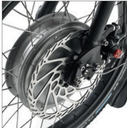
Five hundred watts in the front wheel, two pedals, speeds of up to 28 mph (45 km/h). Sounds straightforward. The difference to other commuting concepts: it actually works and is even loads of fun. The twist-grip throttle on the handlebar lets you control the power coming from the hub motor. You
