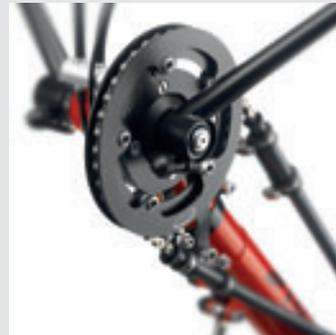
**Hand-crank Assembly: Elbow grease and efficiency**
