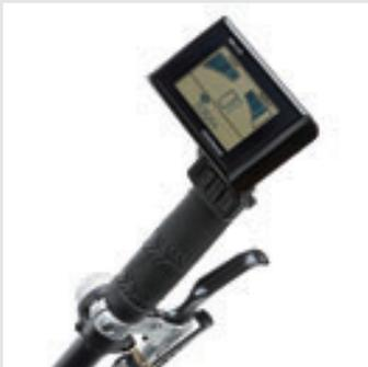
*complete control via the control unit and LCD display: Speed, battery-charge status, assistance level – all route and drive data viewable at a glance; even in sunlight. Easy fingertip operation: you don't even have to take your hand off the grip.*
