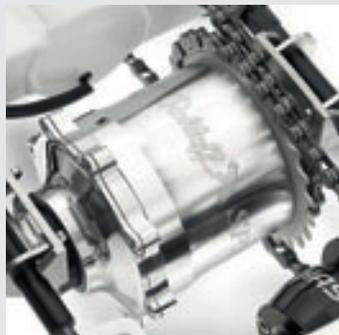
**Rohloff Speedhub:** A true paradigm shift 14 speeds in one high-tech shell: the Rohloff is the best hub on the market: shifts when stationary or under load, extra-wide gear range, even gear spacing, 100% dirt and rain resistant.
