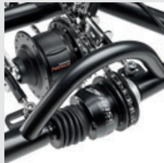
**Differential:** Turns the HANDBIKE into an ATV Specially developed by Marec Hase's team of engineers, the differential transfers the power to both rear wheels – and keeps you going where others throw in the towel, like on steep, gravel paths.
