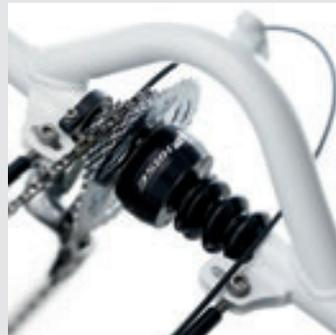
**Differential:** For all-terrain Specially developed by Marec Hase for the KETTWIESEL, the differential guarantees even more riding fun because it transfers the power to both rear wheels. Which can make a world of difference, especially on steep, gravel paths.
