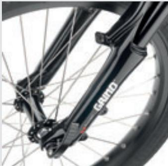
**Spinner Grind I Front Suspension:** Why gallop when you can glide? The optional Spinner suspension fork in its reinforced version (steel shaft) will even satisfy comfort connoisseurs. Forget the pothole slalom: from now on, it's easy gliding over every road.
