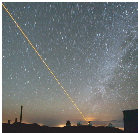
FIGURE 86 Light usually travels in a straight line. In the figure, a sodium frequency laser beam is used as laser guide star to provide a signal for adaptive optics in large telescopes. The laser illuminates a layer of sodium found in the atmosphere at around 90 km of altitude, thus providing an artificial star. The artificial star is used to improve the image quality of the telescope through adaptive optics. In the photograph, the images of the real stars are blurred because of the long exposure time of 3 min (photo Paul Hirst).
