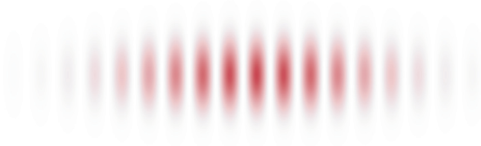
FIGURE 57 Two Gaussian beams interfering at an angle (© Rüdiger Paschotta).
