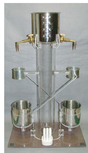
FIGURE 6 A simple Kelvin generator; the one on the right lights a fluorescent light bulb using dripping water (photograph © Harald Chmela).
