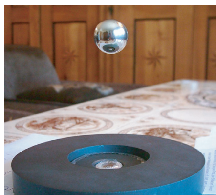
FIGURE 132 Floating 'magic' nowadays available in toy shops, left, with a spinning top and, right, with a spinning magnetic sphere levitating above a large ring magnet (© Kay Kublenz).
