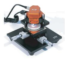
FIGURE 196 The principle and a realization of an atomic force microscope (photograph © Nanosurf).
