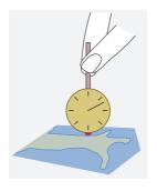
FIGURE 24 A curvimeter or odometer (photograph © Frank Müller).
