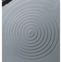
FIGURE 192 An effect of atoms: steps on single crystal surfaces – here silicon carbide grown on a carbon-terminated substrate (left) and on a silicon terminated substrate (right) observed in a simple light microscope (© Dietmar Siche).
