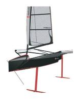
FIGURE 206 The moth sailing class: a 30 kg boat that sails above the water using hydrofoils, i.e., underwater wings (© Bladerider International).
