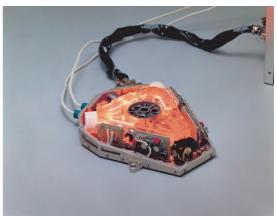
FIGURE 88 The gyroscope: the original system by Foucault with its freely movable spinning top, the mechanical device to bring it to speed, the optical device to detect its motion, the general construction principle, and a modern (triangular) ring laser gyroscope, based on colour change of rotating laser light instead of angular changes of a rotating mass (© CNAM, JAXA).
