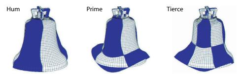
FIGURE 167 The measured fundamental vibration patterns of a bell. Bells – like every other source of oscillations, be it an atom, a molecule, a music instrument or the human voice – show that all oscillations in nature are due to waves. (© H. Spiess & al.).
