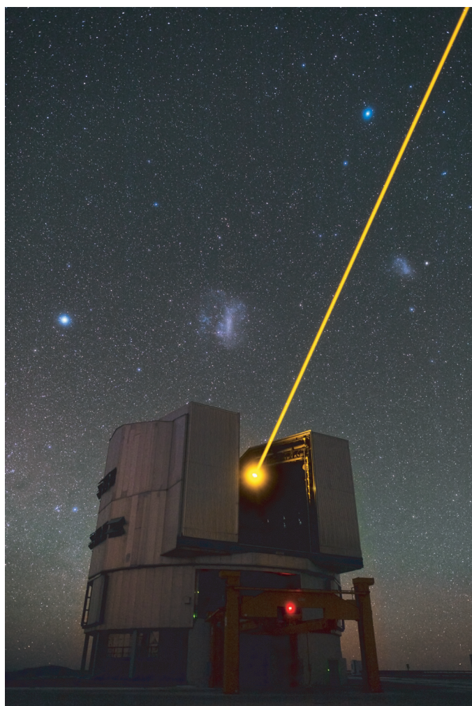
FIGURE 75 The most expensive laser pointer: a yellow 10 W laser that is frequency-stabilized at the wavelength of sodium lamps allows astronomers to improve the image quality of terrestrial telescopes. By exciting sodium atoms found at a height of 80 to 90 km, the laser provides an artificial guide star that is used to compensate for atmospheric turbulence, using the adaptive optics built into the telescope. (© ESO/Babak Tafreshi).
