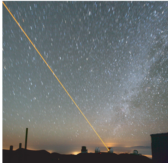
FIGURE 100 Light usually travels in a straight line. In the figure, a sodium frequency laser beam is used as laser guide star to provide a signal for adaptive optics in large telescopes. The laser illuminates a layer of sodium found in the atmosphere at around 90 km of altitude, thus providing an artificial star. The artificial star is used to improve the image quality of the telescope through adaptive optics. In the photograph, the images of the real stars are blurred because of the long exposure time of 3 min (photo by Paul Hirst).
