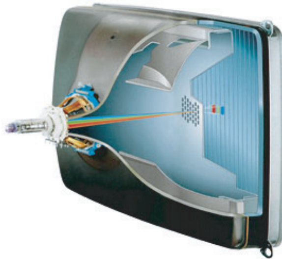
FIGURE 149 A cathode ray tube in older televisions: the first way – now obsolete – to produce changing colour images using electric signals. Television tubes emit an electron beam, deflect it, and generate light by electroluminescence on a coloured screen covered with patterned phosphors.
