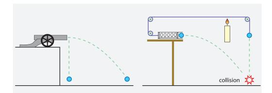
FIGURE 44 Two ways to test that the time of free fall does not depend on horizontal velocity.
