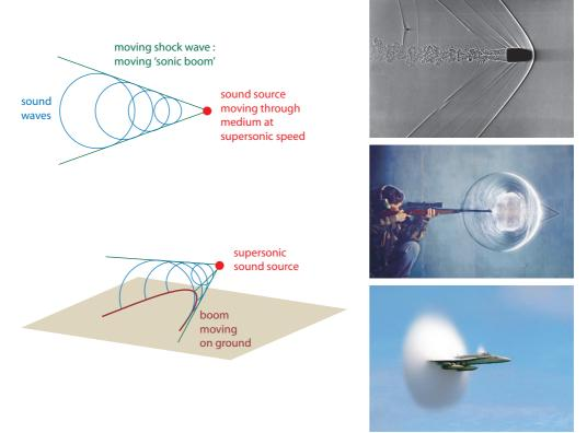
FIGURE 229 The shock wave created by a body in supersonic motion leads to a 'sonic boom' that moves through the air; it can be made visible by Schlieren photography or by water condensation (photo © Andrew Davidhazy, Gary Settles, NASA).
