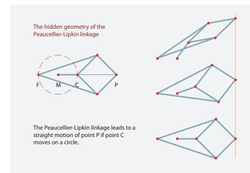
FIGURE 322 How to draw a straight line with a compass (drawn by Zach Joseph Espiritu).
