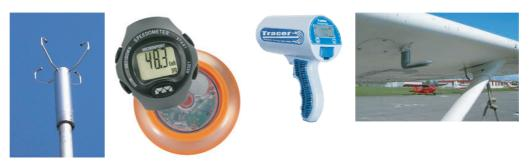
FIGURE 16 Some speed measurement devices: an anemometer, a tachymeter for inline skates, a sport radar gun and a Pitot–Prandtl tube in an aeroplane (© Fachhochschule Koblenz, Silva, Tracer, Wikimedia).
