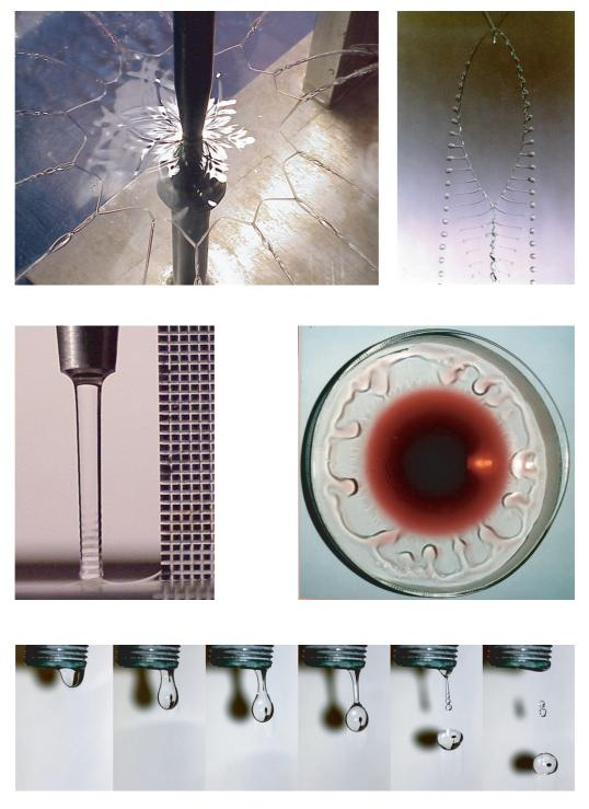
**FIGURE 251** Examples of *laminar* fluid motion: a vertical water jet striking a horizontal impactor, two jets of a glycerol–water mixture colliding at an oblique angle, a water jet impinging on a reservoir in *stationary* motion, a glass of wine showing tears (all © John Bush, MIT) and a dripping water tap (© Andrew Davidhazy).
