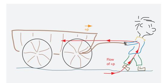
FIGURE 178 The pulling child pumps momentum into the chariot. In fact, some momentum flows back to the ground due to dynamic friction (not drawn).
