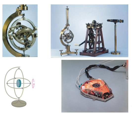
**FIGURE 101** The gyroscope: the original system by Foucault with its freely movable spinning top, the mechanical device to bring it to speed, the optical device to detect its motion, the general construction principle, and a modern (triangular) ring laser gyroscope, based on colour change of rotating laser light instead of angular changes of a rotating mass (© CNAM, JAXA).
