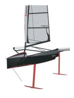
FIGURE 258 The moth sailing class: a 30 kg boat that sails above the water using hydrofoils, i.e., underwater wings (© Bladerider International).
