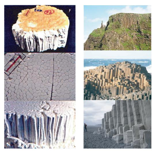
FIGURE 299 A famous correspondence: on the left, hexagonal columns in starch, grown in a kitchen pan (the red lines are 1 cm in length), and on the right, hexagonal columns in basalt, grown from lava in Northern Ireland (top right, view of around 300 m, and middle right, view of around 40 m) and in Iceland (view of about 30 m, bottom right) (© Gerhard Müller, Raphael Kessler - www.raphaelk.co.uk, Bob Pohlad, and Cédric Hüsler).
