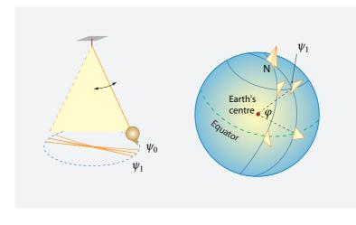
FIGURE 100 The turning motion of a pendulum showing the rotation of the Earth.
