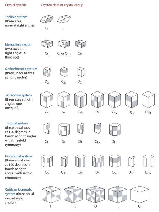
FIGURE 200 The full list of possible symmetries of units cells in crystals, the crystallographic point groups or crystal groups or crystal classes (© Jonathan Goss, after Neil Ashcroft and David Mermin).
