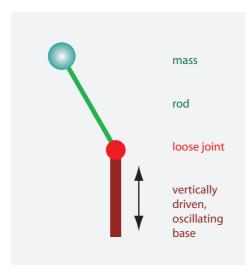
**FIGURE 224** A vertically driven inverse pendulum is stable in the upright position at certain combinations of frequency and amplitude.
