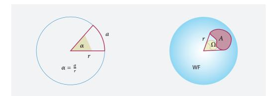
FIGURE 34 The definition of plane and solid angles.
