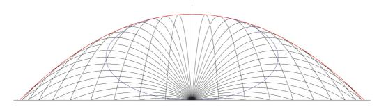
**FIGURE 62** The parabola of safety around a cannon, shown in red. The highest points of all trajectories form an ellipse, shown in blue. (© Theon)
