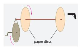
FIGURE 307 A simple way to measure bullet speeds.
