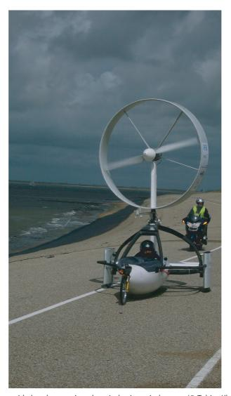
FIGURE 326 A way to ride head-on against the wind using wind power (© Tobias Klaus).
