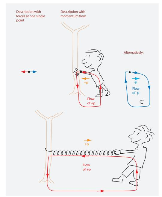
**FIGURE 179** The two equivalent descriptions of situations with zero net force, i.e., with a closed momentum flow. Compression occurs when momentum flow and momentum point in the same direction; extension occurs when momentum flow and momentum point in opposite directions.
