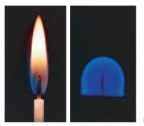
FIGURE 327 A candle on Earth and in microgravity (NASA).
