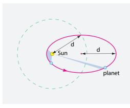
**FIGURE 132** The motion of a planet around the Sun, showing its semimajor axis *d*, which is also the spatial average of its distance from the Sun.
