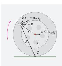
FIGURE 78 The velocities and unit vectors for a rolling wheel.
