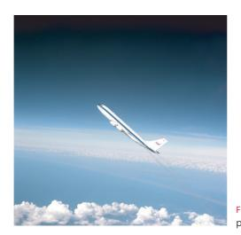
FIGURE 320 The famous 'vomit comet', a KC-135, performing a parabolic flight (NASA).
