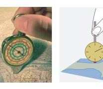
**FIGURE 24** A curvimeter or odometer (photograph © Frank Müller).
