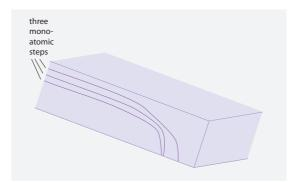
FIGURE 237 Atomic steps in broken gallium arsenide crystals (wafers) can be seen under a light microscope.
