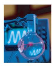
FIGURE 63 Observation of sonoluminescence with a simple set-up that focuses ultrasound in water (© Detlef Lohse).
