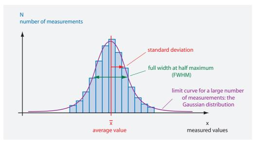
**FIGURE 303** A precision experiment and its measurement distribution. The precision is high if the width of the distribution is narrow; the accuracy is high if the centre of the distribution agrees with the actual value.
