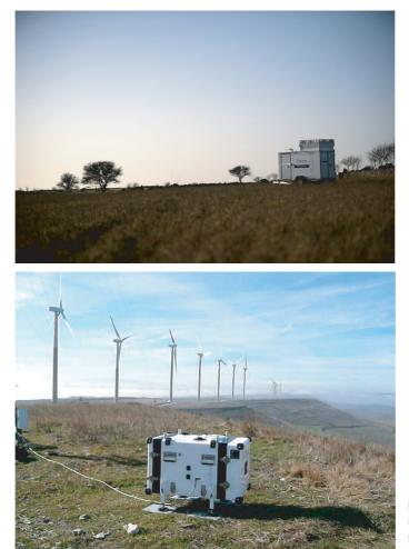
FIGURE 266 Two wind measuring systems: a sodar system and a lidar system (© AQSystems, Leosphere).
