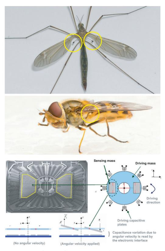
**FIGURE 119** The use of the Coriolis effect in insects – here a crane fly and a hovering fly – and in micro-electromechanic systems (size about a few mm); all provide navigation signals to the systems to which they are attached (© Pinzo, Sean McCann, ST Microelectronics).
