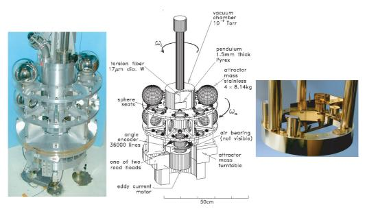
FIGURE 140 A modern precision torsion balance experiment to measure the gravitational constant, performed at the University of Washington (© Eöt-Wash Group).
