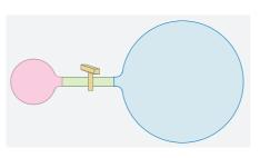
FIGURE 276 Which balloon wins when the tap is opened? Note: this is also how aneurisms grow in arteries.
