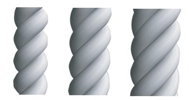
**FIGURE 42** Ideal configurations of ropes made of two, three and four strands. In the ideal configuration, the specific pitch angle relative to the equatorial plane – 39.4°, 42.8° and 43.8°, respectively – leads to zero-twist structures. In these ideal configurations, the rope will neither rotate in one nor in the other direction under vertical strain (© Jakob Bohr).
