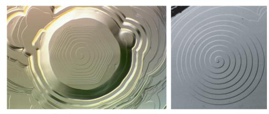
FIGURE 238 An effect of atoms: steps on single crystal surfaces – here silicon carbide grown on a carbon-terminated substrate (left) and on a silicon terminated substrate (right) observed in a simple light microscope (© Dietmar Siche).
