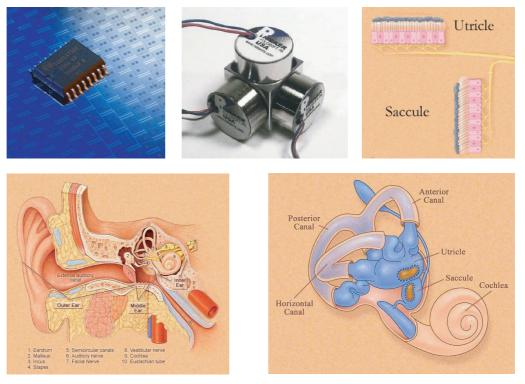
**FIGURE 50** Three accelerometers: a one-axis piezoelectric airbag sensor, a three-axis capacitive accelerometer, and the utricle and saccule near the three semicircular canals inside the human ear (© Bosch, Rieker Electronics, Northwestern University).
