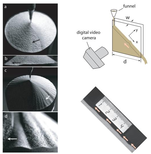
**FIGURE 287** Examples of self-organization for sand: spontaneous appearance of a temporal cycle (a and b), spontaneous appearance of a periodic pattern (b and c), spontaneous appearance of a spatiotemporal pattern, namely solitary waves (right) (© Ernesto Altshuler et al.).
