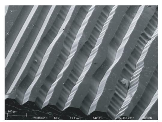
**FIGURE 207** The centre of the grooves in an old vinyl record show the amplitude of the sound pressure, averaged over the two stereo channels (scanning electron microscope image by © Chris Supranowitz/University of Rochester).
