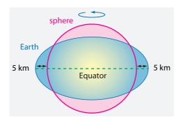
**FIGURE 96** Earth's deviation from spherical shape due to its rotation (exaggerated).
