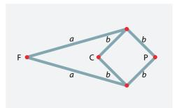
FIGURE 185 A famous mechanism, the *Peaucellier-Lipkin linkage*, consists of (grey) rods and (red) joints and allows drawing a straight line with a compass: fix point F, put a pencil into joint P, and then move C with a compass along a circle.
