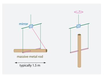
FIGURE 106 Observing the rotation of the Earth in two seconds.
