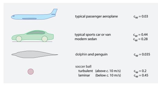
FIGURE 181 Shapes and air/water resistance.
