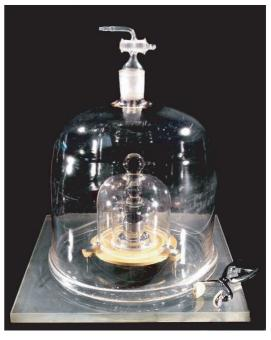
FIGURE 66 The standard kilogram (until 2019) (© BIPM).
