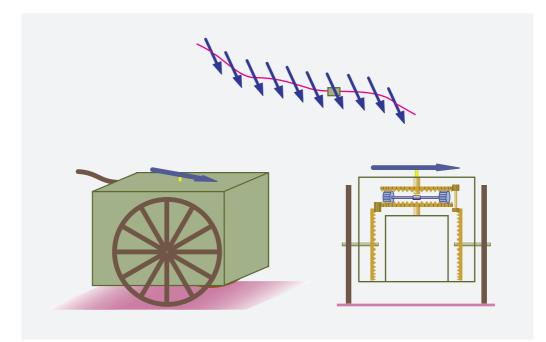
FIGURE 323 The mechanism inside the south-pointing carriage.
