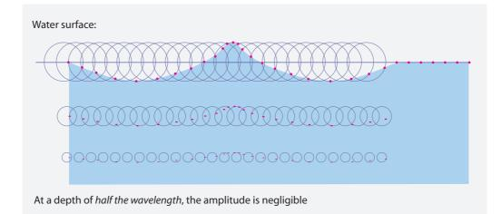
**FIGURE 208** The formation of the shape of deep gravity waves, on and under water, from the circular motion of the water particles. Note the non-sinusoidal shape of the wave.
