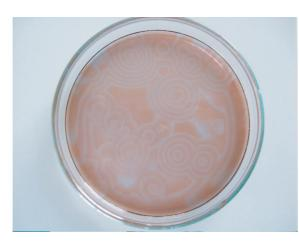
FIGURE 298 The Belousov-Zhabotinski reaction: the liquid periodically changes colour, both in space and time (© Yamaguchi University).
