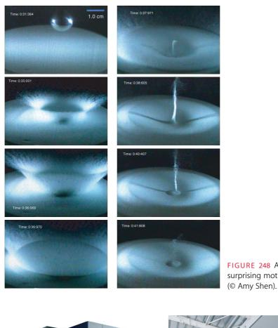
FIGURE 248 An example of a surprising motion of sand: granular jets (© Amy Shen).
