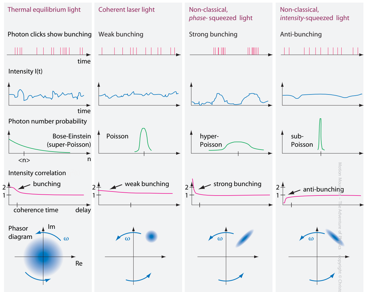
FIGURE 21 Four types of light and their photon properties: thermal light, laser light, and two extreme types of non-classical, squeezed light.
