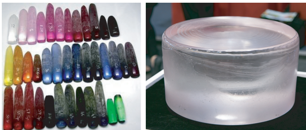
FIGURE 35 Left: raw crystals, or boules, of synthetic corundum, picture size c. 50 cm. Right: a modern, 115 kg corundum single crystal, size c. 50 cm (© Morion Company, GT Advanced).
