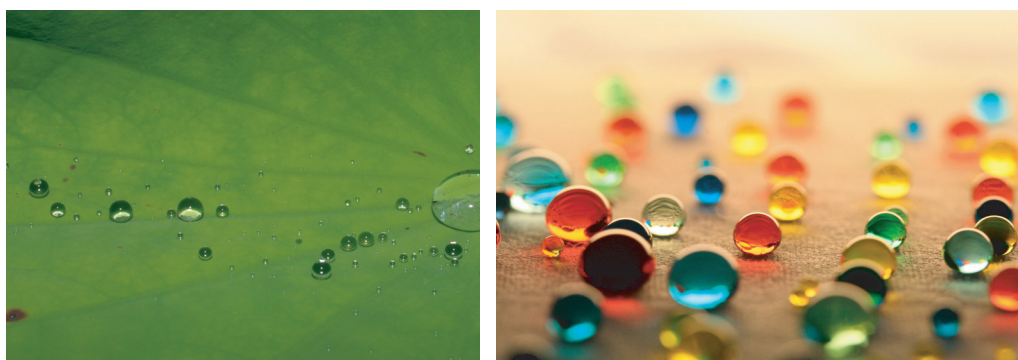
FIGURE 66 The beauty of materials science: the surface of a lotus leaf leads to almost spherical water droplets; plasma-deposited PTFE, or teflon, on cotton leads to the same effect for the coloured water droplets on it (© tapperboy, Diener Electronics).
