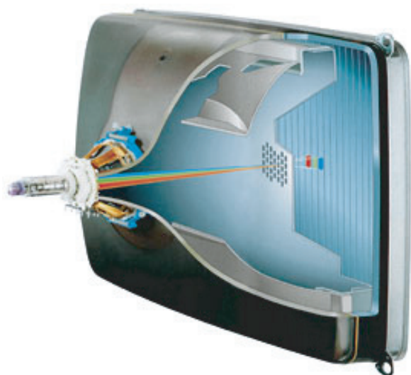
FIGURE 148 A cathode ray tube in older televisions: the first way – now obsolete – to produce changing colour images using electric signals. Television tubes emit an electron beam, deflect it, and generate light by electroluminescence on a coloured screen covered with patterned phosphors.
