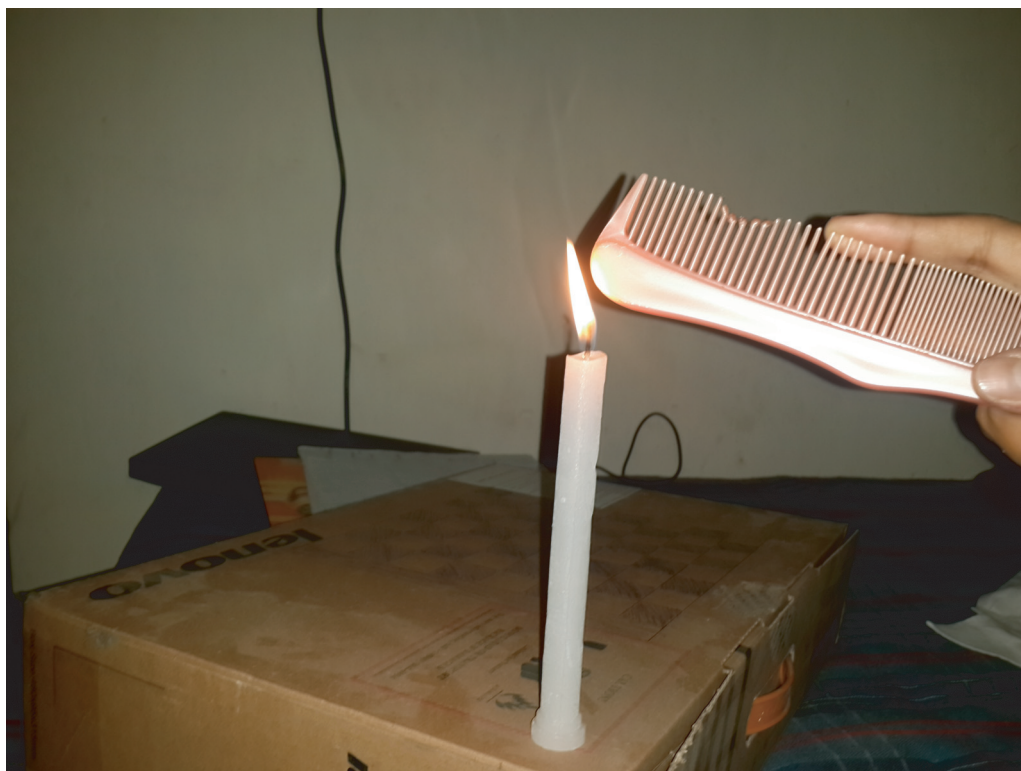
FIGURE 186 The way a flame reacts to a rubbed comb (© Shubham Das and Rakesh Kumar).
