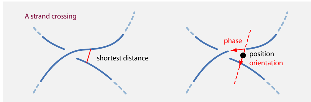
FIGURE 12 The definition of a crossing, its position, its orientation and its phase. The shortest distance defines a local density.
