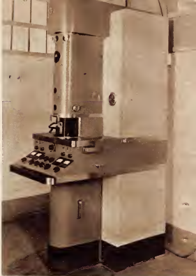
A different RCA-made type of electron microscope, a perfected form of something that started out as a whole laboratory full of busy apparatus.
