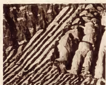
Another sample of pearlite from eutectoid steel, also at 10,000 times.
