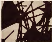
Mingled crystals of metallic zinc and zinc oxide at 10,000 times life size.
