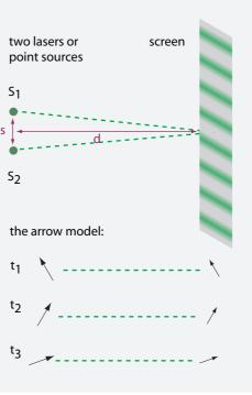
FIGURE 30 Interference and the description of light with arrows (at three instants of time).
