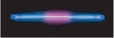
FIGURE 78 A low-pressure hydrogen discharge in a 20 cm long glass tube (© Jürgen Bauer at www. smart-elements.com).
