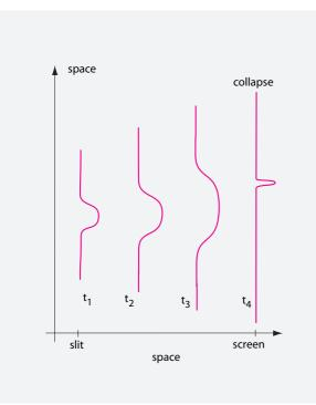
FIGURE 73 Quantum mechanical motion: an electron wave function (actually its module squared) from the moment it passes a slit until it hits a screen
