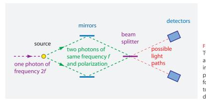
FIGURE 58 Two-photon emission and interference: two indistinguishable photons are always found arriving together, at the same detector.
