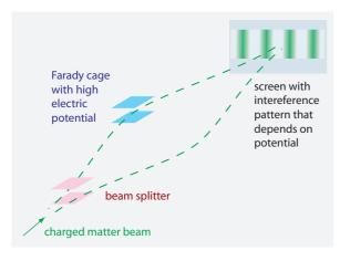
FIGURE 49 A localized electric potential in an interferometer leads to a shift of the interference pattern.
