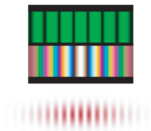
FIGURE 29 Top: calculated interference patterns – and indistinguishable from observed ones under ideal, "textbook" conditions - produced by two parallel narrow slits illuminated with green light and with white light. Bottom: two Gaussian beams interfering at an angle (© Dietrich Zawischa, Rüdiger Paschotta).
