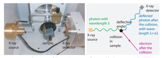
FIGURE 20 A modern version of Compton's experiment fits on a table. The experiment shows that photons have momentum: X-rays - and thus the photons they consist of - change frequency when they hit the electrons in matter in exactly the same way as predicted from colliding particles (© Helene Hoffmann).
