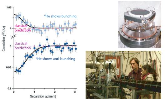
FIGURE 59 Bunching and antibunching of <sup>3</sup>He and <sup>4</sup>He helium!bunching atoms: the measurement result, the detector and the experiment (from atomoptic.iota.u-psud.fr/research/helium/helium.html, photo © Denis Boiron, Jerome Chatin).
