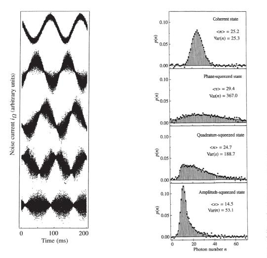
FIGURE 90 Left, from top to bottom: the electric field and its fuzziness measured for a coherent state, for a squeezed vacuum state, for a phase-squeezed state, for a mixed, quadrature-squeezed state and for an amplitude-squeezed state, all with a small number of photons. Right: the corresponding photon number distributions for the uppermost four states. (© G. Breitenbach/Macmillan, from Ref. 19)
