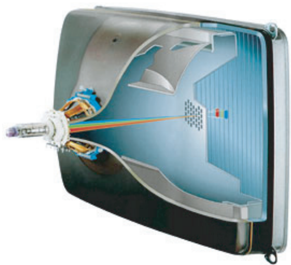
FIGURE 146 A cathode ray tube in older televisions: the first way – now obsolete – to produce changing colour images using electric signals. Television tubes emit an electron beam, deflect it, and generate light by electroluminescence on a coloured screen covered with patterned phosphors.
