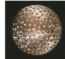
FIGURE 74 The LAGEOS satellites: metal spheres with a diameter of 60 cm, a mass of 407 kg, and covered with 426 retroreflectors (courtesy NASA).
