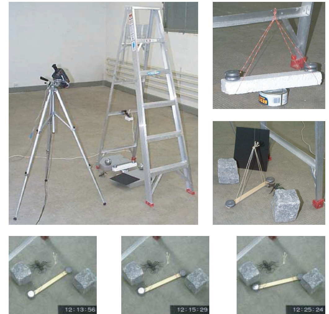
FIGURE 139 Home experiments that allow determining the gravitational constant G , weighing the Earth, proving that gravity also works sideways and showing that gravity curves space. Top left and right: a torsion balance made of foam and lead, with pétanque (boules) masses as fixed masses; centre right: a torsion balance made of wood and lead, with stones as fixed masses; bottom: a time sequence showing how the stones do attract the lead (© John Walker).
