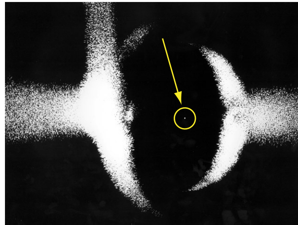
FIGURE 239 A single barium ion levitated in a Paul trap (image size around 2 mm) at the centre of the picture, visible also to the naked eye in the original experiment, performed in 1985 (© Werner Neuhauser).
