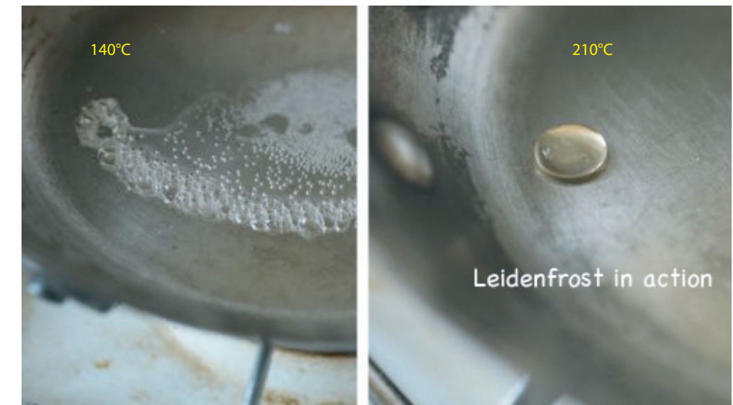
FIGURE 267 A water droplet on a pan: an example of the Leidenfrost effect (© Kenji Lopez-Alt).
