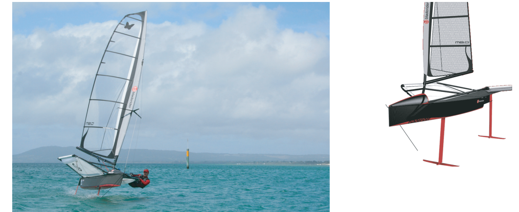
FIGURE 258 The moth sailing class: a 30 kg boat that sails above the water using hydrofoils , i.e., underwater wings (© Bladerider International).
