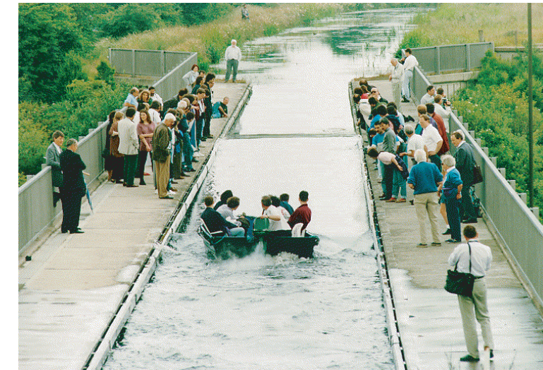
FIGURE 222 A solitary water wave followed by a motor boat, reconstructing the discovery by Scott Russell (© Dugald Duncan).
