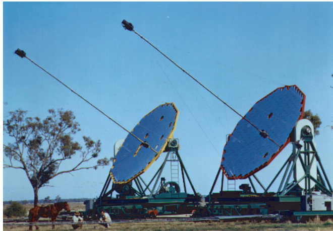
FIGURE 24 The original experimental set-up with which Hanbury Brown and Twiss measured stellar diameters at Narrabri in Australia. The distance between the two light collectors could be changed by moving them on rails. The light detectors are at the end of the poles and each of them, as they wrote, ‘collected light as rain in a bucket.’ (© John Davis).
