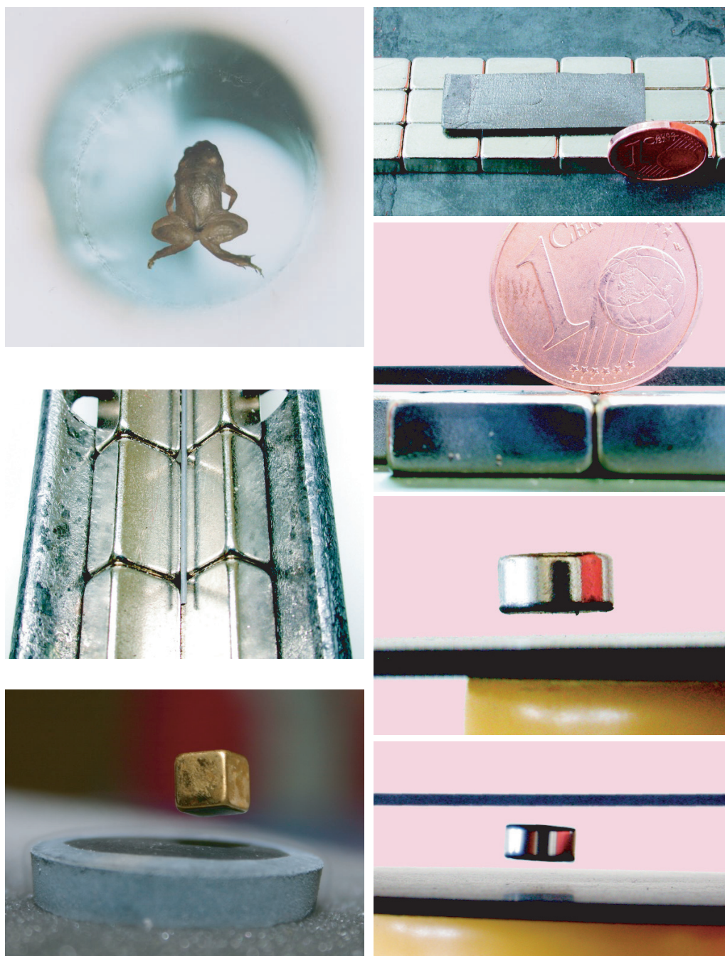
FIGURE 169 Stable diamagnetic levitation. Left: a living frog in a 16 T magnet, a graphite bar over rectangular permanent magnets, and a brass-coloured magnet over a superconducting ring. Right: two levitating graphite plates, one seen from above and another from the side; below, levitation of a 4 mm diameter NdFeB permanent magnet, above a graphite plate and between two graphite plates, near a large ring magnet that is not shown (© Lijnis Nelemans, Peter Nussbaumer, and Joachim Schlichting from Ref. 179).
