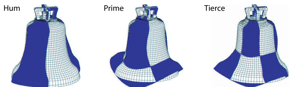
FIGURE 206 The measured fundamental vibration patterns of a bell. Bells – like every other source of oscillations, be it an atom, a molecule, a music instrument or the human voice – show that all oscillations in nature are due to waves. (© H. Spiess & al.).
