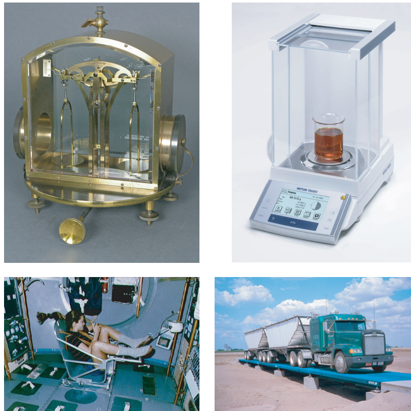
FIGURE 71 Mass measurement devices: a vacuum balance used in 1890 by Dmitriy Ivanovich Mendeleyev, a modern laboratory balance, a device to measure the mass of a cosmonaut in space and a truck scales (© Thinktank Trust, Mettler-Toledo, NASA, Anonymous).
