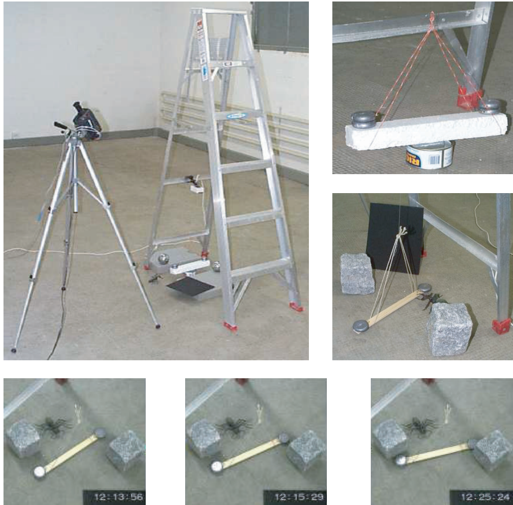
FIGURE 139 Home experiments that allow determining the gravitational constant G , weighing the Earth, proving that gravity also works sideways and showing that gravity curves space. Top left and right: a torsion balance made of foam and lead, with pétanque (boules) masses as fixed masses; centre right: a torsion balance made of wood and lead, with stones as fixed masses; bottom: a time sequence showing how the stones do attract the lead (© John Walker).
