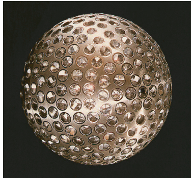
FIGURE 76 The LAGEOS satellites: metal spheres with a diameter of 60 cm, a mass of 407 kg, and covered with 426 retroreflectors (courtesy NASA).
