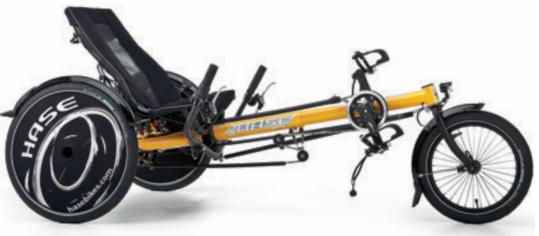
easy one: significantly more stability than conventional rehab trikes, excellent maneuverability, a high level of active safety thanks to the disc brakes on the rear wheels, and easy operation. In no time at all, it can be ergonomically adjusted to any rider from 4'1" to 6'3" (1.25-1.90 m) in height. What luck that the HASE BIKES designers still had a few TRIX up their sleeves!
