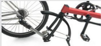
Tow Bar: Follow me! Lame name, fine piece of equipment: with the Tow Bar, even standard bikes can be used as towing vehicles for the KETTWIESEL – with a safety bonus: the integrated overrun brake works automatically. When the towing bike brakes, the KETTWIESEL brakes.
