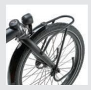
Lowrider Rack: Low and be held More touring luggage: our Lowrider Rack puts more weight on the front wheel without affecting the handling. The advantage over standard lowrider racks: mounts behind the seat-back. The low plenty of clearance between the panniers and the pedals! (Not compati- KETTWIESEL even more solid in the
