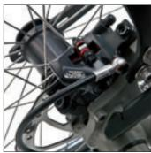
Tektro brakes: Smooth and crisp The hydraulic Tektro Auriga Twin on the KLIMAX rear wheels offer superior modulation. But they can also bite down hard if the need arises. One brake lever controls the two discs on the rear wheels. Low maintenance included.
