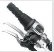
Single-hand Controls: Join forces A single grip with all control elements! Using a special adapter, two brake levers can be mounted on one side. This allows the rider to shift gears and control both brake levers using a single hand.
