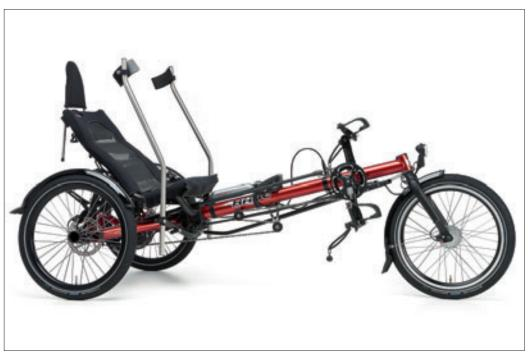
Special Steering / Shoulder Steering Unit: Twist and turn Mobility for people with no arms or short arms. The width of the steering unit is fully adjustable. A coaster brake is used for stopping, and the Shimano Nexus automatic hub gears, for shifting.
