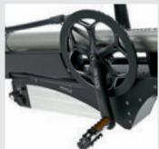
Additional Battery: Energy bar Double your mileage with motor assistance? No problem. The additional rechargeable lithium-ion power pack has more weight onto the front wheel withthe same properties as the standard battery. The extra 9 pounds (4 kg) are a piece of cake for the KLIMAX 5K. And one more energy bar never hurt.
