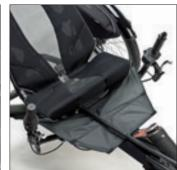
Splash Guard: Dry duds, dude! It turns the KLIMAX 5K into a true all-weather sprinter: your trousers stay dry, even when the path is peppered with puddles. It also keeps dirt and moisture away from the drive train - which reduces maintenance requirements.
