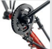
Elbow grease and efficiency For people with a disability, it's often the only option for self-propelled mobility. The HASE BIKES Hand-crank Assembly can be folded forward for easy mounting and dismounting and has incredible torsional stiffness as well as excellent efficiency.
