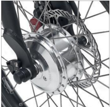
Electric Motor: The power pack For long and hilly commutes or just a little extra speed and comfort: the Protanium motor transforms the LEPUS into a trike hybrid. The 250 W package on the front wheel powers along when you start pedaling. Otherwise it travels incognito—in hub disguise.
